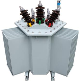
S13 type three-phase coil iron core distribution transformer capacity range 30-2500KVA. The iron core is a three-phase three-column coil structure with internal and external frame. High degree of mechanization, lamination coefficient is large. The high and low pressure coils are wound continuously on the core column, the concentricity is good, and the coils are tight. The main technical and economic indicators have reached the international advanced level of the same kind of products.
