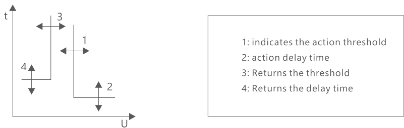
Figure 2 Action principle of overvoltage protection
