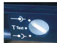
In the "Connect" position, the main circuit and All secondary circuits are connected
