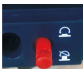
In "separate", "test", "connect" In three positions, the position lock is locked, and the crank cannot Operation (locked state)
