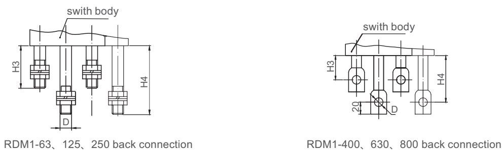
Fig 8 RDM1-63~800 Back connection overall and installation dimension
