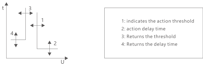
Figure 2 Action principle of overvoltage protection
