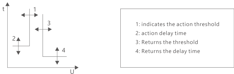
Figure 1 Action principle of undervoltage protection
