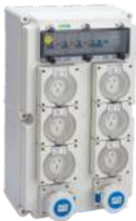
Model No: DTG001 Dimension: 300×160×500mm(H,W,D) 6×3P 15A waterproof socket 2×3P 16A CEE waterproof socket
