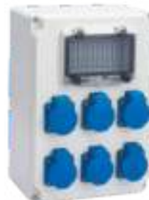
Model No DTG006 Dimension: 300×160×400mm 6×16A IP44 IEC Socket and MCB(RCD)
