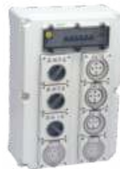
Model No: DTG003 Dimension:350×180×530mm 2×5P 32A waterproof socket and switch 1×5P 20A waterproof socket and switch 2×3P 15A waterproof socket
