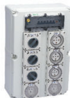
Model No: DTG003 Dimension: 350X180X530mm 2X5P 32A waterproof socket and switch 1X5P 20A waterproof socket and switch 2X3P 15A waterproof socket
