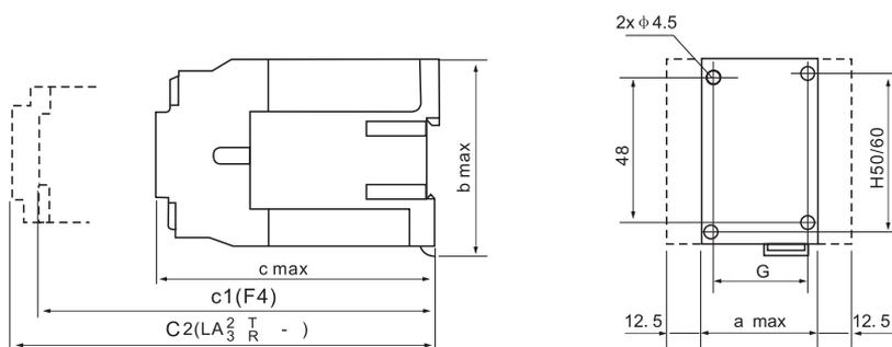
Note: C: CJX2-Z; C1: CJX2-Z+F4; C2: CJX2-Z+LA2-D/LA3-D -CJX2-09Z/12Z/18Z
