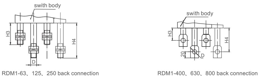
Fig 8 RDM1-63~800 Back connection overall and installation dimension
