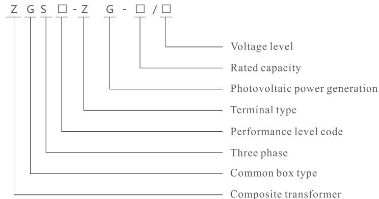
Scheme 2: PV pre-installed substation (China transformer structure) Rated capacity (KVA)
